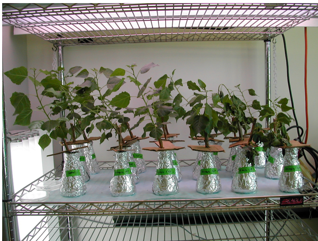
Figure 2-2 Hybrid poplar cuttings with increasing concentrations of TNT from left to right (in units of \text{mg L}^{-1} ): 0, 4, 6, 8, 10, and 20.
